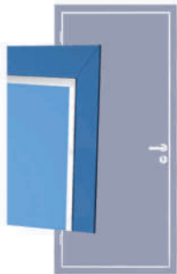
The lines of door leaf ends surrounded stainless steel "U" shaped profile.
