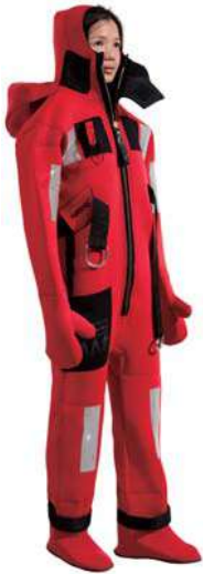
HXF-9 儿童保温服 面料材质: 氯丁橡胶 产品浮力: ≥90N 保温性能: 在0℃ - +2℃ 平静水流中历史6小时, 体温降低不超过2℃, 配有 救生衣灯、口哨、伙伴绳和提拉带 HXF-9 CHILDREN IMMERSION SUIT Fabric Material: Neoprene Product floating: ≥90N Insulation properties: At 0℃ - +2℃ history 6 hours in calmwater , hypothermia does not exceed 2℃, with a life jacket lights, whistles , partners rope and pulling loop .
