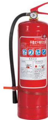
MFZ/ABC 8kg 干粉灭火器 外径: 164mm 最大工作压力: 1.2Mpa 环境温度: -20℃~+55℃ 测试压力: 2.1Mpa 最小壁厚: ≥2.5mm 材质: 碳钢 灭火等级: 4A144B 采用标准: CCS/ZY/EC MFZ/ABC 8kg POWDER FIRE EXTINGUISHER Diameter: 164mm Maximum working pressure: 1.2Mpa Ambient temperature: -20℃~+55℃ Test pressure: 2.1Mpa Minimum wall thickness: ≥2.5mm Material: Carbon Steel Fire Rating: 4A144B Standard: CCS / ZY / EC
