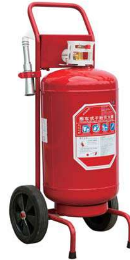
MFZ/ABC 35kg 推车式干粉灭火器 外径: 325mm 最大工作压力: 1.2Mpa 环境温度: -20℃~+55℃ 测试压力: 2.1Mpa 最小壁厚: ≥3.8mm 材质: 碳钢 灭火等级: 6A183B 采用标准: CCS/ZY/EC MFZ/ABC 35kg WHEELED POWDER FIRE EXTINGUISHER Diameter: 325mm Maximum working pressure: 1.2Mpa Ambient temperature: -20℃~+55℃ Test pressure: 2.1Mpa Minimum wall thickness: ≥3.8mm Material: Carbon Steel Fire Rating: 6A183B Standard: CCS / ZY / EC
