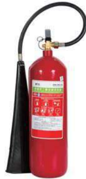
MT/5 CO 2 灭火器5kg 外径: 155mm 最大工作压力: 17Mpa 测试压力: 25Mpa 最小壁厚: ≥3.0mm 材质: 合金钢 灭火等级: 34B 采用标准: CCS/ZY/EC MT/5 CO 2 FIRE EXTINGUISHER 5kg Diameter: 155mm Maximum working pressure: 17Mpa Test pressure: 25Mpa Minimum wall thickness: ≥ 3.0mm Material: Steel Fire Rating: 34B Standard: CCS / ZY / EC
