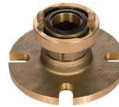
HXXF-21国际通岸接头 材质：黄铜 工作压力：0.1Mpa 螺栓和螺母：M16*50mm*4根 接口规格：DN50/DN65 认证：CCS/ZY HXXF-21 INTERNATIONAL SHORE CONNECTION Material: Brass Working pressure: 0.1Mpa Bolts and nuts: M16 * 50mm * 4 Specification: DN50/DN65 Certificate: CCS/ZY
