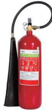
MT/7 CO 2 灭火器7kg 外径: 155mm 最大工作压力: 17Mpa 测试压力: 25Mpa 最小壁厚: ≥3.4mm 材质: 合金钢 灭火等级: 55B 采用标准: CCS/ZY/EC MT/7 CO 2 FIRE EXTINGUISHER 7kg Diameter: 155mm Maximum working pressure: 17Mpa Test pressure: 25Mpa Minimum wall thickness: ≥ 3.4mm Material: Alloy Steel Fire Rating: 55B Standard: CCS / ZY / EC
