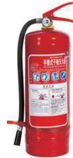
MFZ/ABC 5kg 干粉灭火器 外径: 150mm 最大工作压力: 1.2Mpa 环境温度: -20℃~+55℃ 测试压力: 2.1Mpa 最小壁厚: ≥1.3mm 材质: 碳钢 灭火等级: 3A89B 采用标准: CCS/ZY/EC MFZ/ABC 5kg POWDER FIRE EXTINGUISHER Diameter: 150mm Maximum working pressure: 1.2Mpa Ambient temperature: -20℃~+55℃ Test pressure: 2.1Mpa Minimum wall thickness: ≥1.3mm Material: Carbon Steel Fire Rating: 3A89B Standard: CCS / ZY / EC
