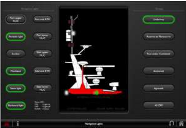
Navigation and signal lantern control and monitoring.
